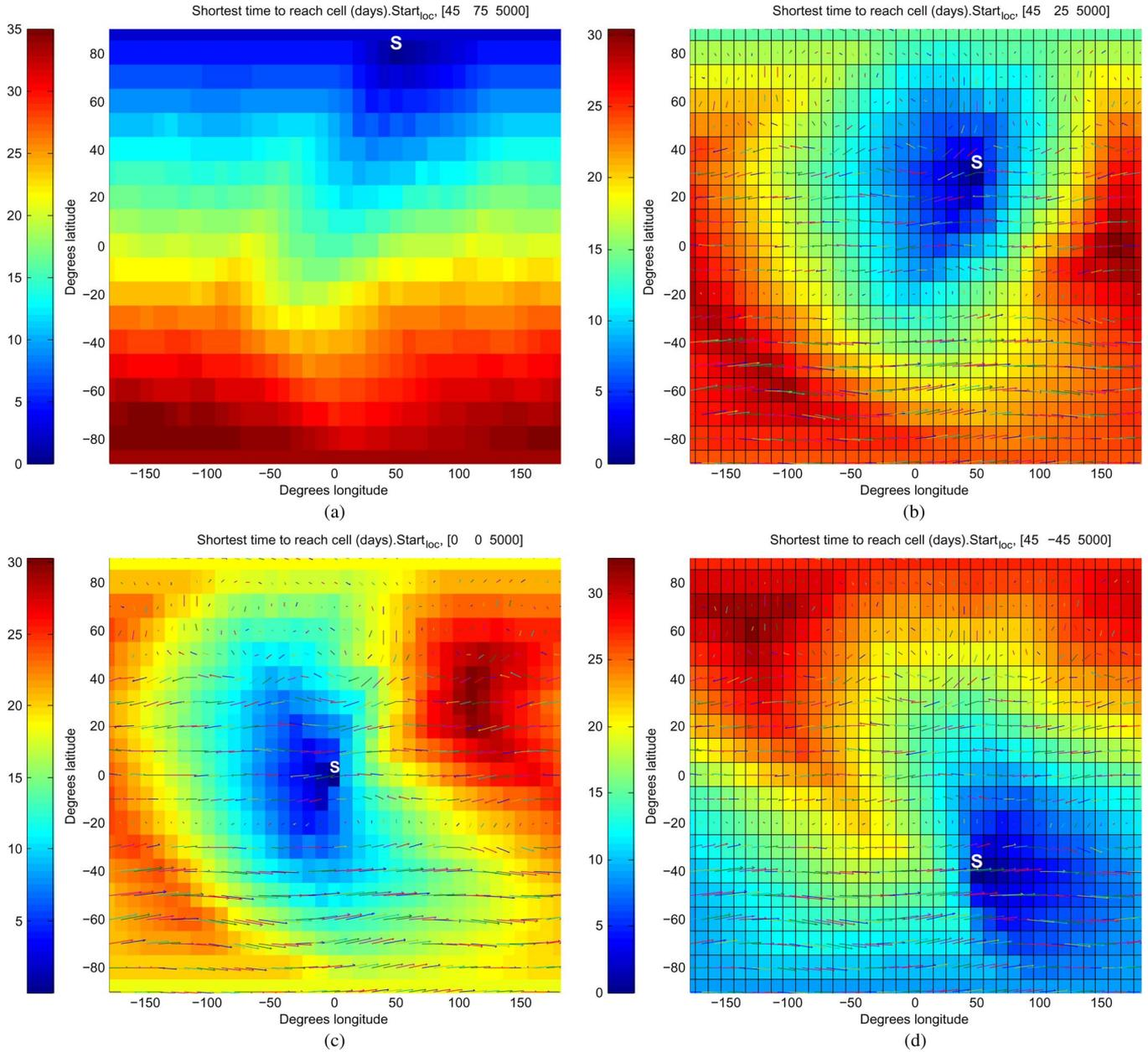
Fig. 5. Global reachability map with 1 m/s horizontal actuation and static wind field. (a) From 90° N, 45° E. (b) From 25° N, 45° E. (c) From 0° N, 0° E. (d) From 45° S, 45° E.
