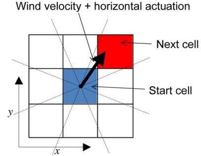
Fig. 2. Discretization in the horizontal plane.
