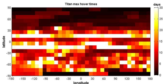
Fig. 13. Titan wind field maximum hover times within each latitude and longitude cell, for the case of no horizontal actuation. Grid resolution of  $10^\circ \times 10^\circ \times 500$  m, altitude up to 10 km, static wind field at time  $L_s = 0^\circ$ .
