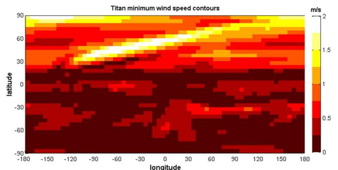
Fig. 12. Titan wind field minimum magnitudes at each latitude and longitude, over altitude up to 10 km, binned to 0.25-m/s intervals. Grid resolution of  $5^\circ \times 5^\circ \times 500$  m, with static wind field at time  $L_s = 0^\circ$ .
