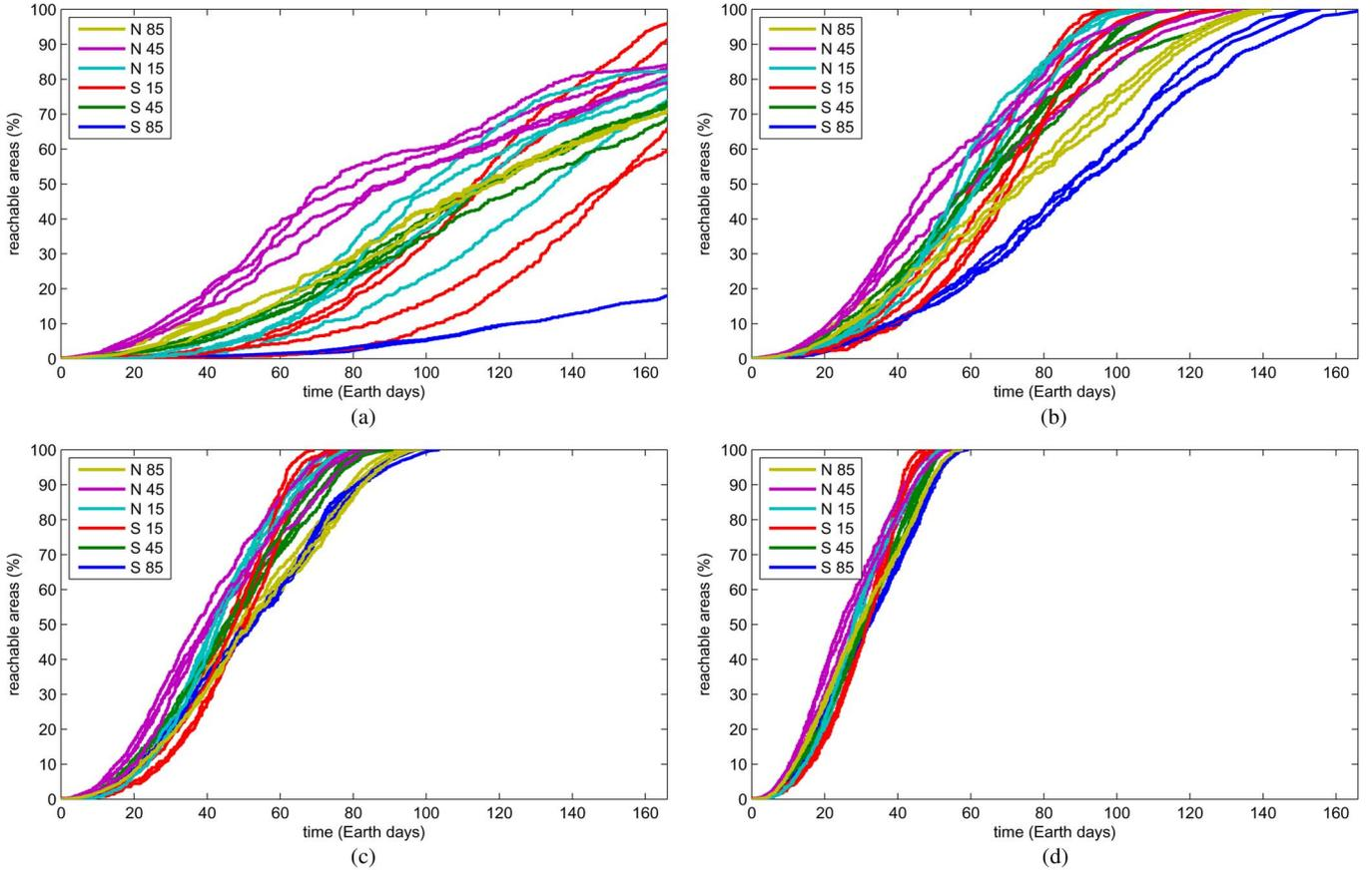
Fig. 8. Percentage of reachable area given a starting location.  $L_s = 0^\circ$ . (a) 0.0-m/s horizontal actuation. (b) 0.25-m/s horizontal actuation. (c) 0.50-m/s horizontal actuation. (d) 1.0-m/s horizontal actuation.
