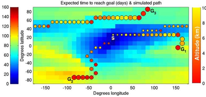
Fig. 7. Trajectories from a start to three different goals ( $G_1$ ,  $G_2$ , and  $G_3$ ). Trajectories are marked with circles whose color represents the altitude. The corresponding color bar is given at the right. The left color bar shows the time to reach each cell at an altitude of 250 m (in Earth days).
