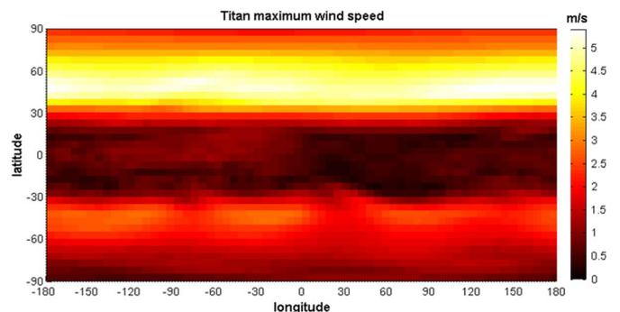
Fig. 11. Titan wind field maximum magnitudes at each latitude and longitude, over altitude up to 10 km. Grid resolution of  $5^\circ \times 5^\circ \times 500$  m, with static wind field at time  $L_s = 0^\circ$ .
