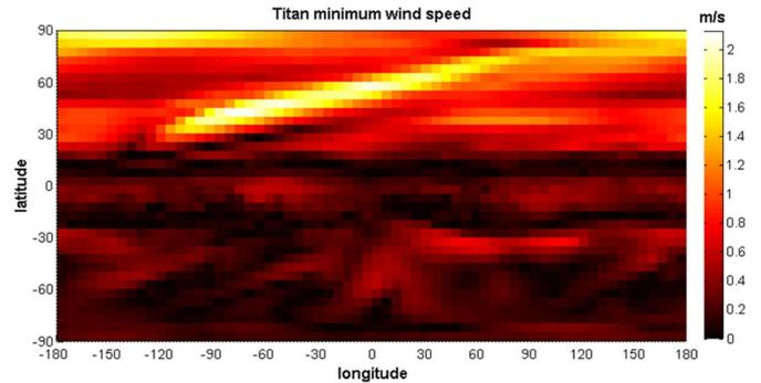
Fig. 10. Titan wind field minimum magnitudes at each latitude and longitude, over altitude up to 10 km. Grid resolution of  $5^\circ \times 5^\circ \times 500$  m, with static wind field at time  $L_s = 0^\circ$ .
