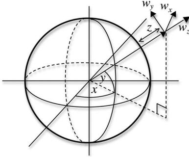
Fig. 1. Coordinate frame definitions. Degrees longitude is denoted by  $x$ , degrees latitude is denoted by  $y$ , and  $z$  is the altitude from the surface of the planet. Velocities  $w_x$ ,  $w_y$ , and  $w_z$  are defined in a Cartesian coordinate frame fixed to the local surface tangent.
