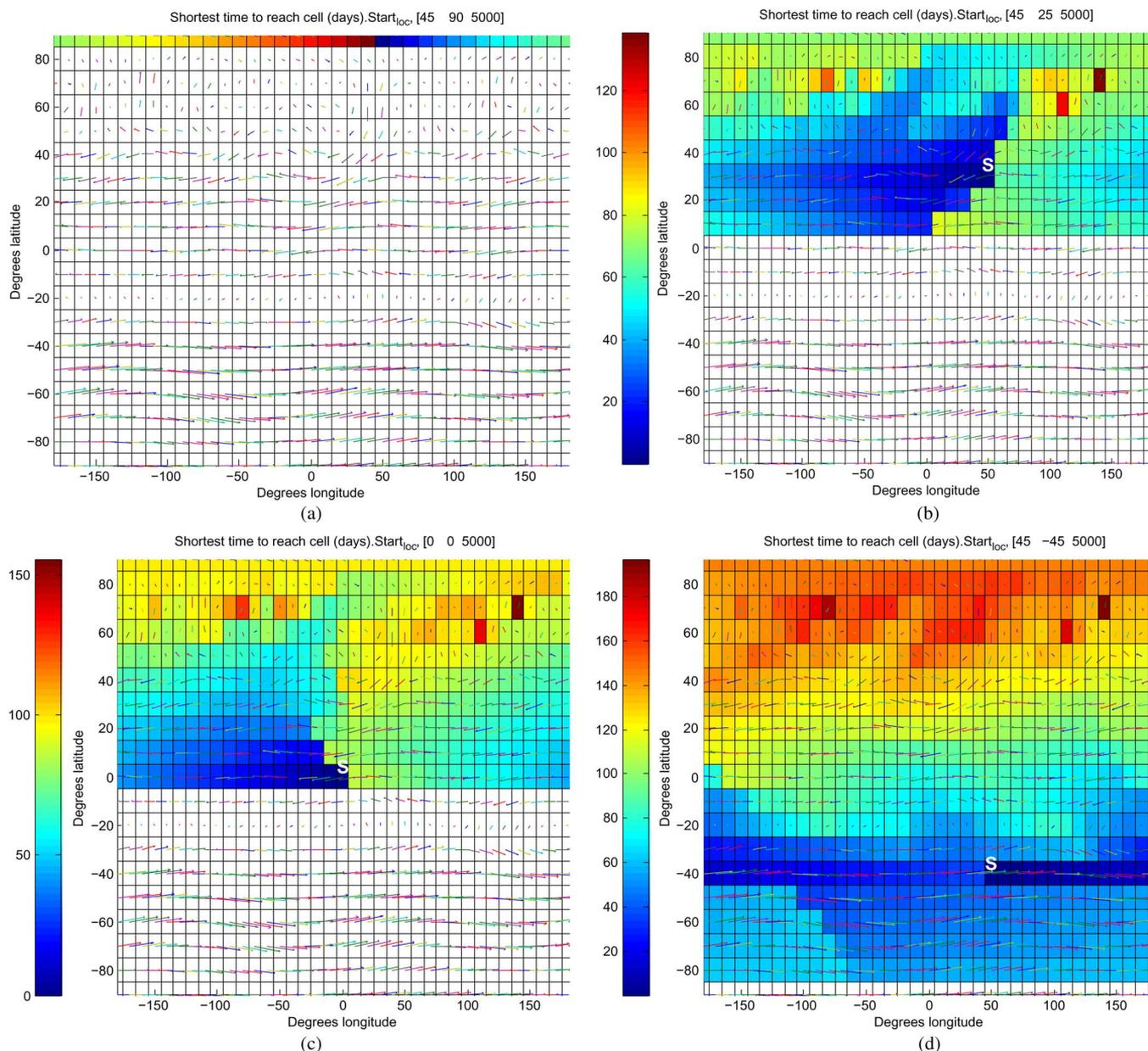
Fig. 4. Global reachability map with no horizontal actuation and static wind field. (a) From 90° N, 45° E. (b) From 25° N, 45° E. (c) From 0° N, 0° E. (d) From 45° S, 45° E.
